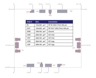
Eutectic Die bond using AuSn (80/20) solder is recommended.
