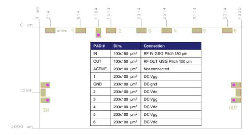
Eutectic Die bond using AuSn (80/20) solder is recommended.
