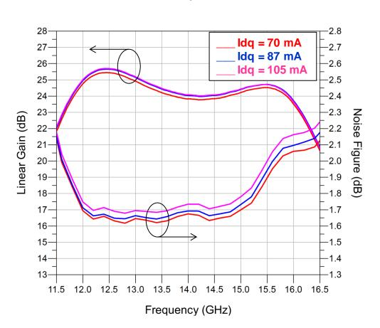
Test Conditions:  $T_{base_plate} = 25^{\circ}C$ , Vd = 15 V
