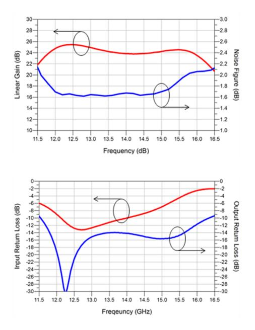
Test Conditions:  $T_{base_plate} = 25^{\circ}C$ , Vd = 15 V, Idq = 70 mA
