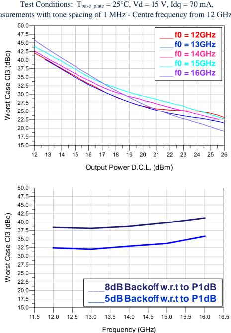
2-tone measurements with tone spacing of 1 MHz - Centre frequency from 12 GHz to 16 GHz
