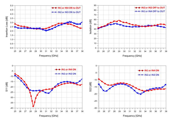
Test Conditions: Tbase\_plate = 25°C - CW, 0/-2V Control Voltages
