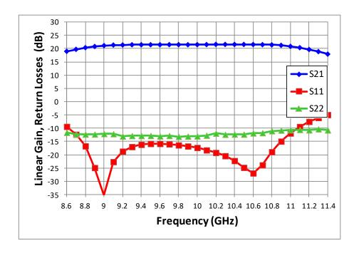
Test Conditions:  $T_{base\_plate} = 25^{\circ}C$ , Vd = 6 V, Idq = 190 mA - Input Power = 7 dBm
